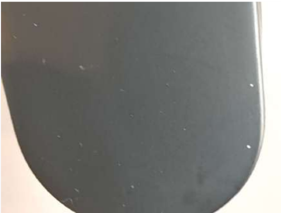
Ref # 20.4 - Mixer has paint splatter
